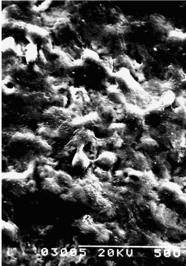
Figure 19 SEM of piled up FBGCs at the bottom of large crater of the large surface roughness, SB-4HF 120.
